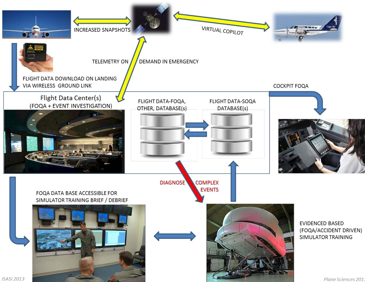
Following the data flow from the top left and going counterclockwise:
