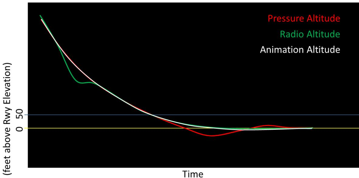
However, this assumes that the aircraft *is above the runway elevation at 50 feet*. If for example, the aircraft lands short and there is a valley before the runway threshold, this method will not work as the valley will result in an increase in height that will show the aircraft rising when it did not as shown in the yellow line in the figure.
