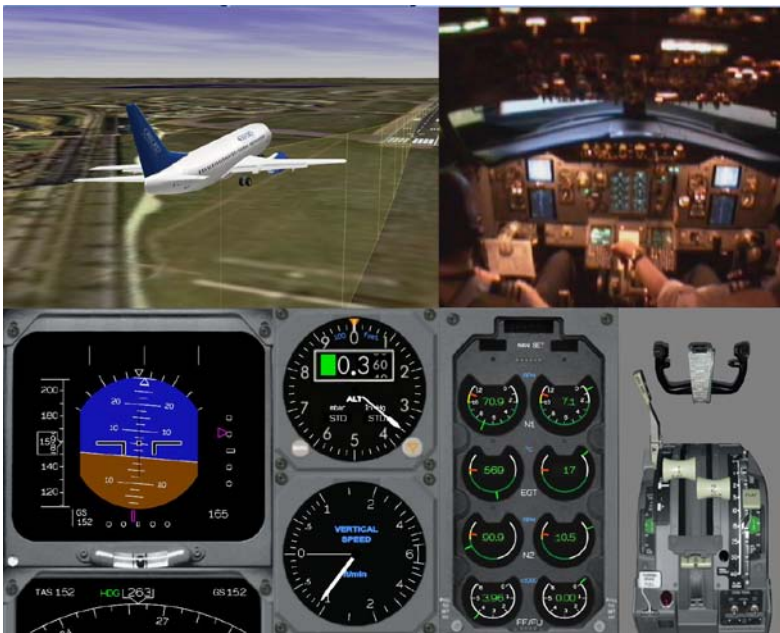
Figure 6: Simulator session animation replay using same core technology as accident investigation replay (Courtesy Oxford Aviation).
